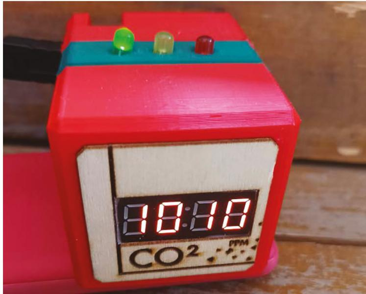
Figure 5.18: Finalised sensor showing CO<sub>2</sub> level. Credit: FAB.
