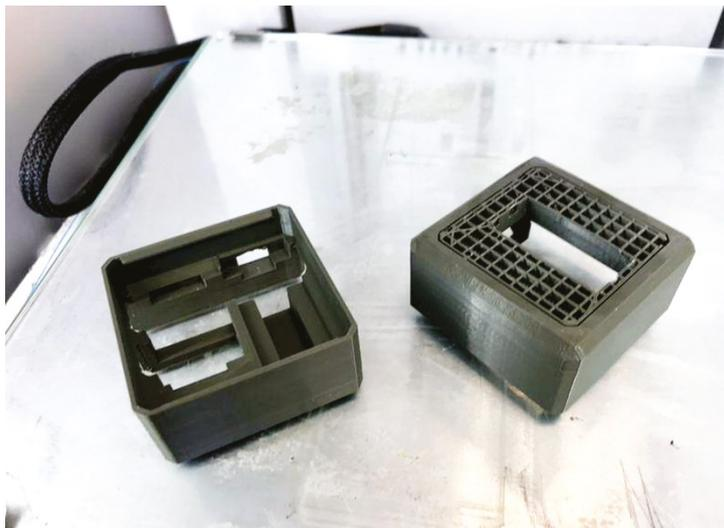
Figure 5.13: 3D printed sensor box. Credit: FAB.
