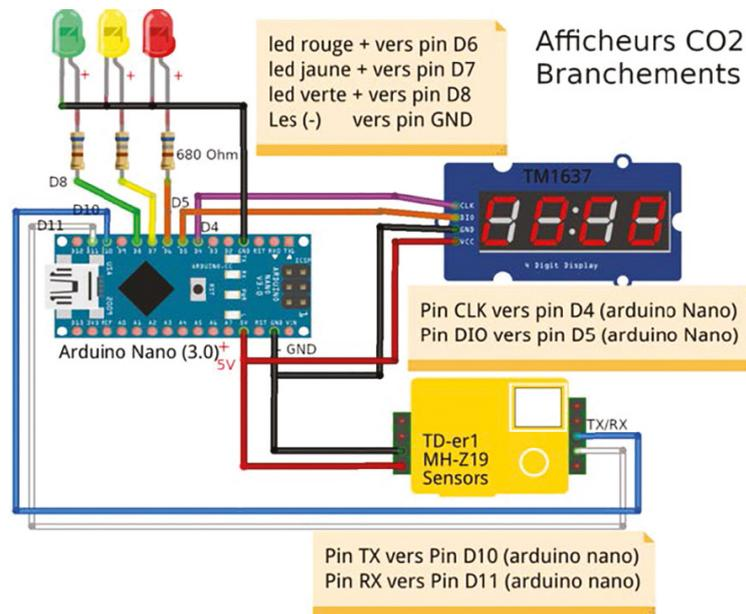
Figure 5.16: Overview of connections [French]. Credit: FAB.
