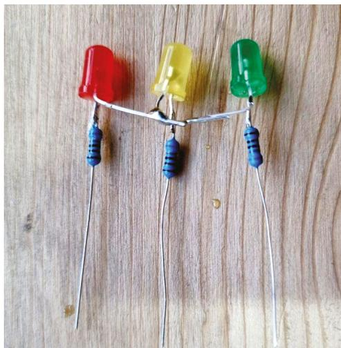
Figure 5.15: Soldered LEDs and Ohm resistors. Credit: FAB.
