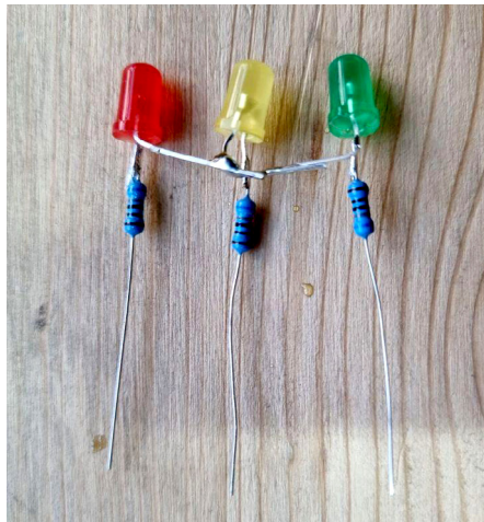
Figure 20: Soldered LEDs and Ohm resistors. Credit: FAB.
