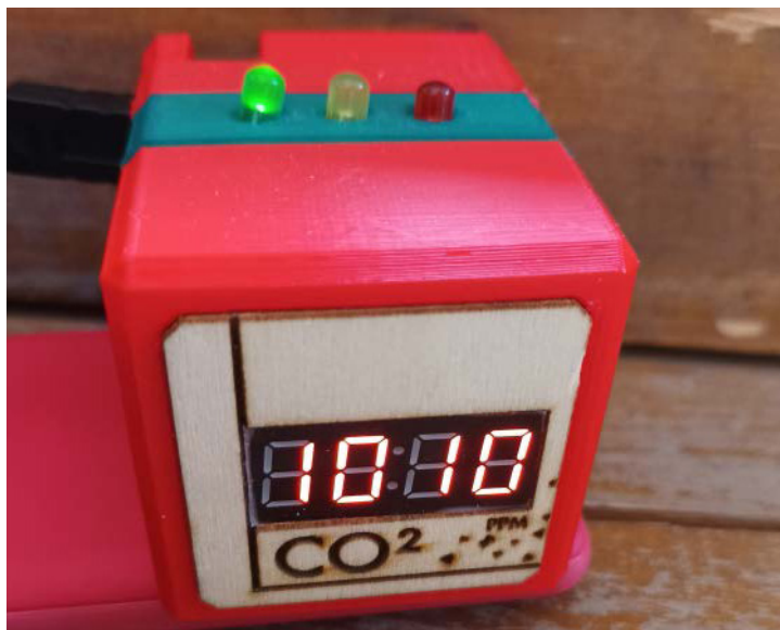
Figure 22: Finalised sensor showing CO 2 level. Credit: FAB.
